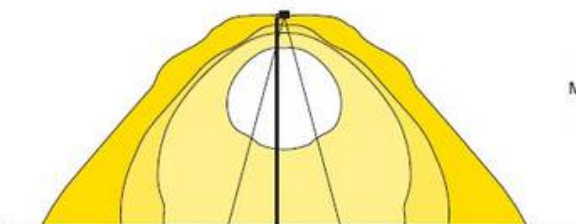
Metal Halide Floodlight - 400W 7 x 6 Wide Distribution (0° Tilt)
